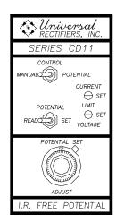
1. Manual-Potential switch must be in manual position.
